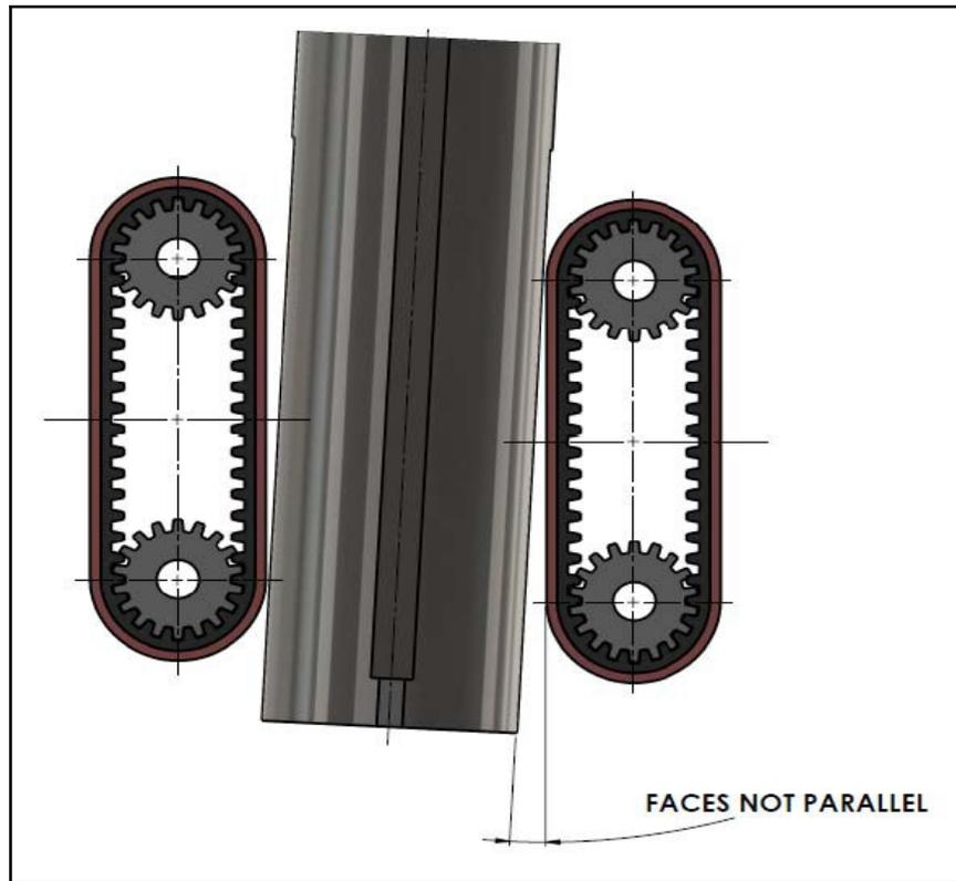
**Fig 3:** Example of tube misalignment.
