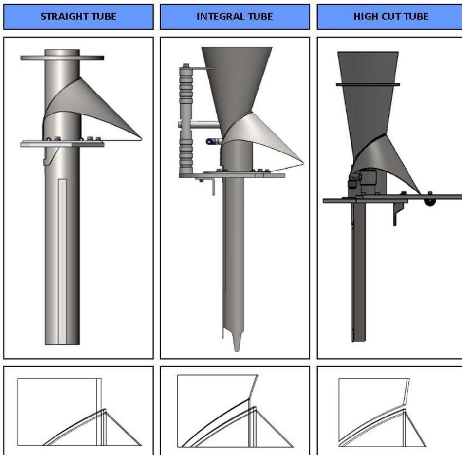
**Fig 2:** Various tube inlet design options.
