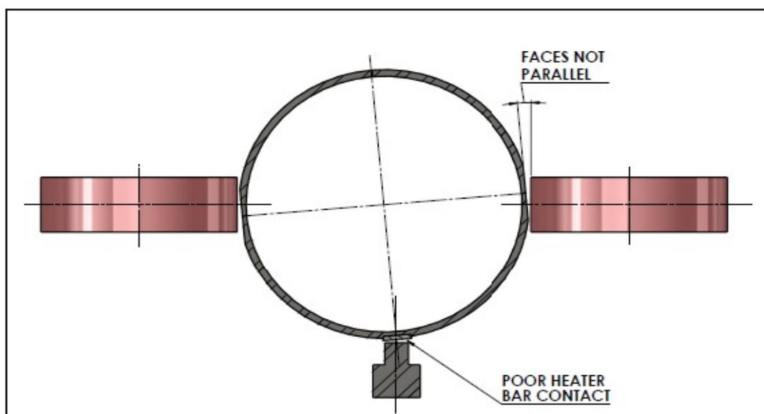
Fig 4: Example of tube twist.
